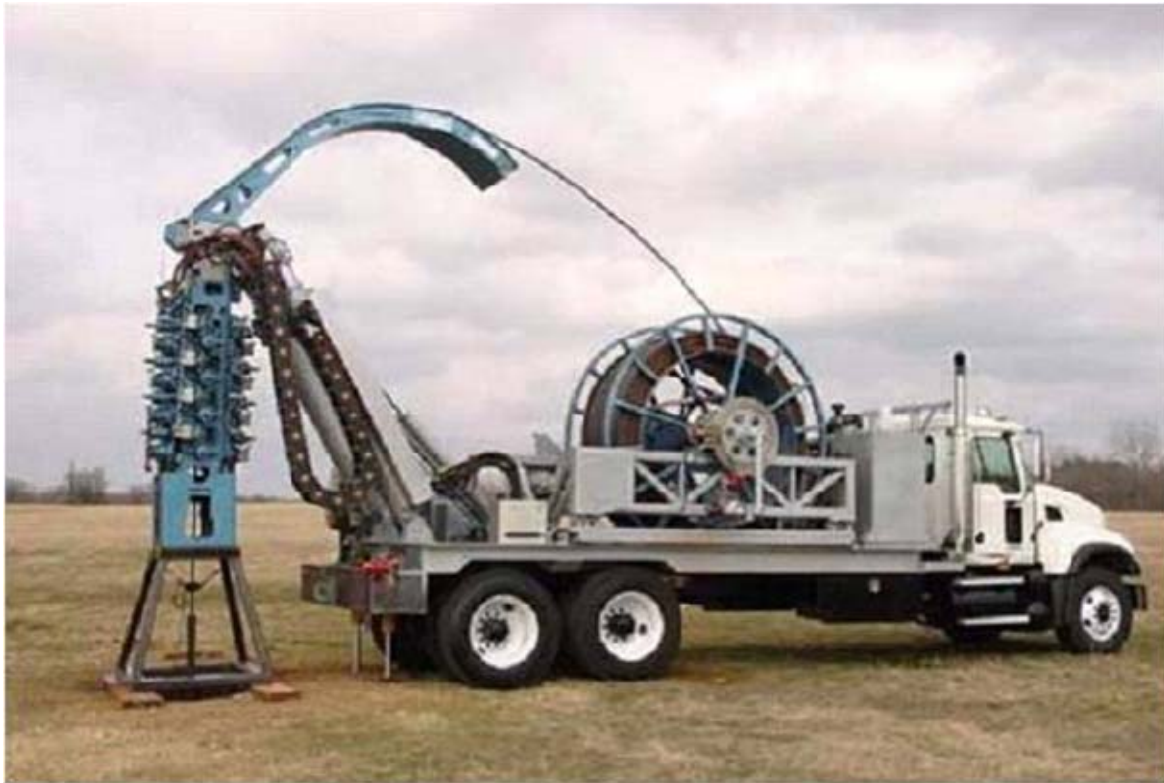
Figure 1. Coiled tubing rig on location.
